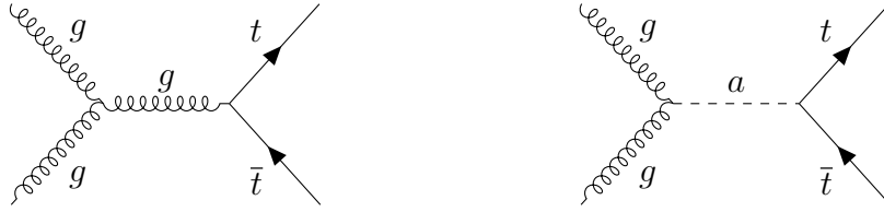
Figure 4.1: Feynman diagrams for t\bar{t} production with the s-channel Standard Model process (left) and the ALP process (right).
